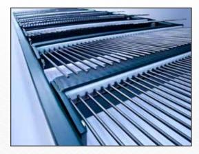
Kleenskreen™ Finger Deck System is made for difficult-to-screen material where blinding, clogging, matting, and pegging cause problems with traditional screening media. The Kleenskreen™ can be retrofitted to existing portable and stationary screening plants, giving the producer a viable and very economic choice of not having to purchase a new piece of equipment similar to a StarScreen or trommel.
